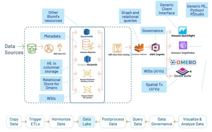
The solution architecture is being developed to enable ETL of all metadata, data, and results from various sources for efficient querying, visualization, and analysis. iji
